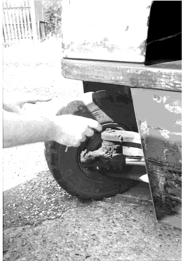
Kingpin greased with Lofrix Grease
